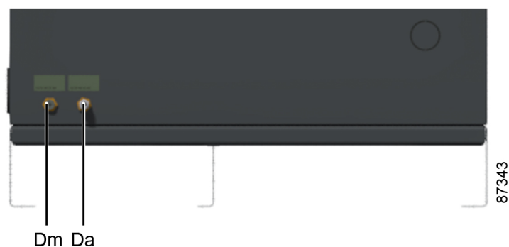
Figure 14: Condensate drain connections, Pack
