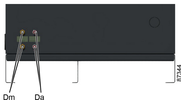
Figure 15: Condensate drain connections, Full-Feature
