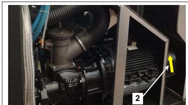
Direction of rotation fixed speed and VSD.
