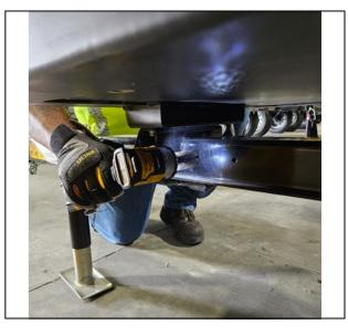
6. Ensure that jack-stand clevis pin is properly installed before starting this task. Raise jack so drawbar can swing to vertical position freely, be cautious of pinch points exposed when drawbar is rotated 90 degrees.
