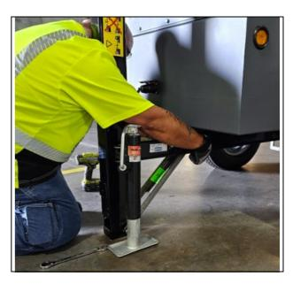
12.Place bolt retrieved from step 10 through the lower hole of the drawbar and shipping bracket. Hand tighten nut.
