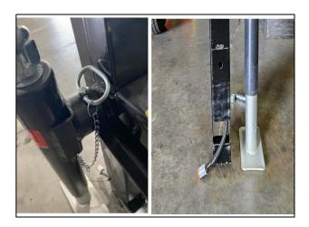
7. Once draw bar is 90 degrees perpendicular to the floor, lower jack until both the bottom of the tow bar and jack are resting on flat level ground.
