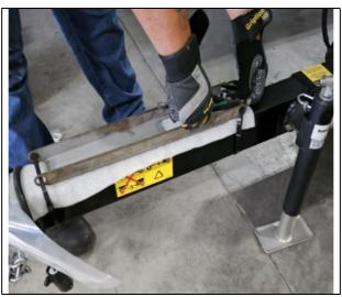
5. Remove rear bolt on tow bar with wrench and impact socket.
