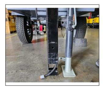
8. Insert latch pin into 1/2" hole to mechanically prevent the drawbar from rotating back into tow position.
