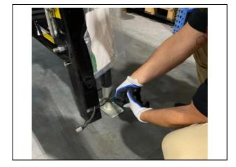
15.Completed drawbar secured in upright position, ready for shipping.
