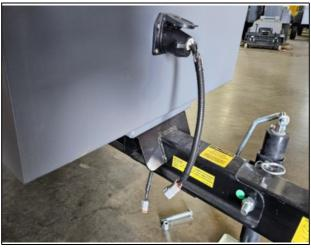
4. Use wire cutters or scissors to cut zip ties which secure the shipping bracket in place.
